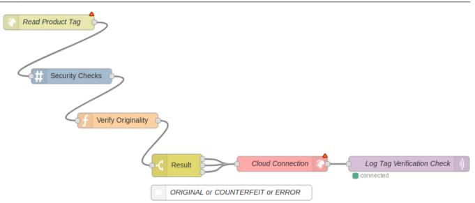
FIGURE 3 Node-RED Flow - Product's originality tag verification
